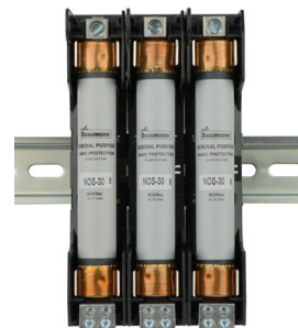
600 volt 30 amp modular blocks with single port lineside lugs and four port loadside lugs.
