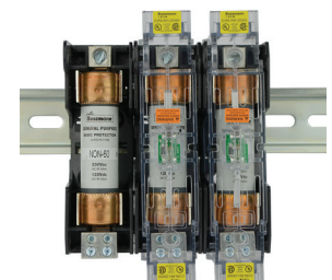
250 volt 60 amp modular blocks with single port lineside lugs and four port loadside lugs with optional finger-safe IP20 covers.
