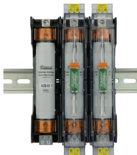
600 volt 60 amp modular blocks with single port lineside lugs and four port loadside lugs and optional finger-safe IP20 covers.
