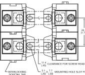
BLOCK NO. 1BS101 This block is furnished with an interlocking dovetail feature as shown. When mounting multiple fuseblocks side by side, center-to-center distance between mounting holes each pole is 44.58 (1.755).
