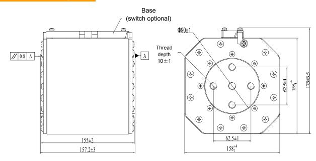
Note: Coaxiality of both ends of contact 0.8mm
