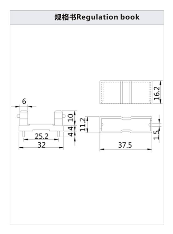
With integral protection against electric shock. Fuse-holders shall have live parts inaccessible to IEC 529 1mm diameter rigid test wire when fully assembled, without fuse carrier or fuse in place and when fuse carrier, with fuse is being inserted or withdrawn.
