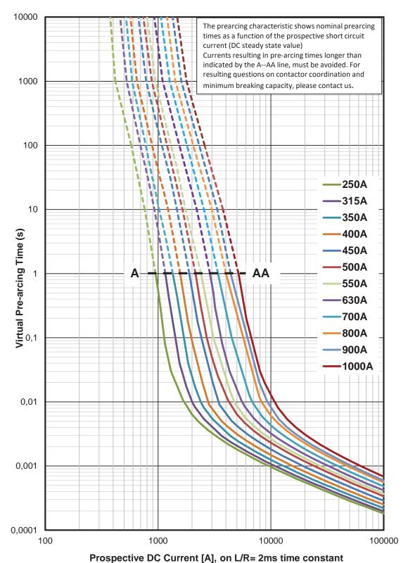
Pre-production and sample electric vehicle square body fuse links, 500 V d.c. 250 to 1000 Amps, fuse body sizes 1\* to 2
