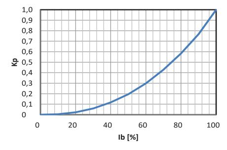
$\mbox{Ib}:\mbox{R.M.S.}$  value of load current as % of rated current Kp: correction factor for power loss
